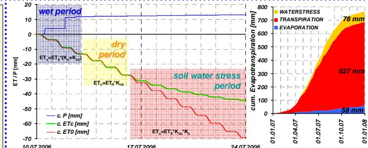
Measurement of grass evapotranspiration ( $ET_c$  adj.) using a precise weighing monolithic lysimeter show the effect of plant water availability depending on specific soil conditions.
