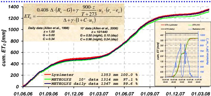
Results comparison over long time observation periods show a very good agreement between measured grass ETc at HYDROLYS – Lysimeter results and calculated METEOLYS  $ET_0$  on a daily data base (deviation of the sum over 22 month = 0.4 %). 10' data calculation of daily sum of ETc better reflects the influence of changing weather conditions during the day. This effect is shown for July, 10' 2007 where a thunderstorm about noon reduces evapotranspiration rates.
